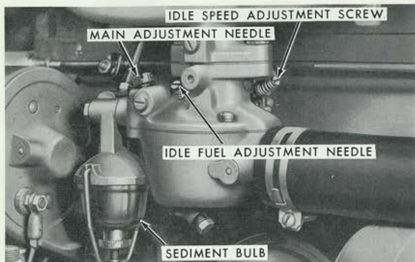
Figure 32 Adjusting the Carburetor (Series 2000)
