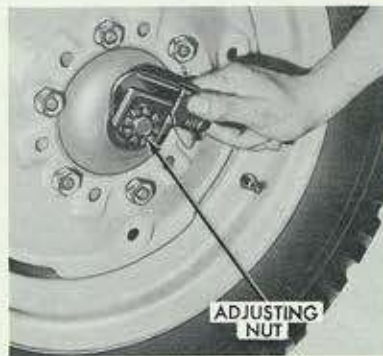
Figure 46 Adjusting Front Wheel Bearings
