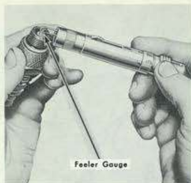
Figure 42 Checking Spark Plug Gap
