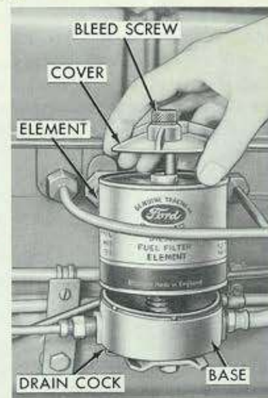
Figure 25 Replacing Diesel Fuel Filter
